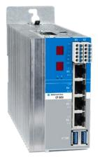
with 2 Ethernet 2 VARAN, 1 CAN 2 USB 2.0 (Type A), 1 USB 3.2 (Type C) 1 DisplayPort, 1 S-DVI
