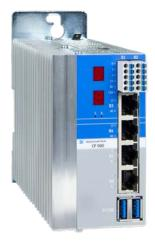
with 2 Ethernet 2 VARAN, 1 CAN 2 USB 3.2 (Type A), 1 USB 3.2 (Type C) 1 DisplayPort
